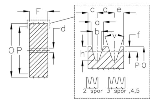
$\begin{array}{ll} d & = 15 \\ F & = 50.0 \\ Number of ribs = 3 \\ O & = 90.5 \\ P & = 85 \\ Type & = A \end{array}$
